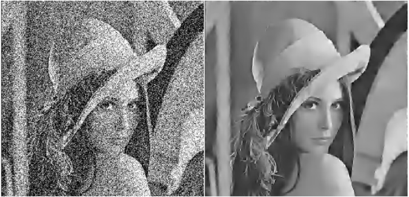
Fig. 6. Optimal denoising method applied to noisy “Lena” image. Left: Corrupted image \tilde{f}(x, y) , \sigma_n = 50 , PSNR = 14.16 dB. Right: Optimally denoised image \hat{f}^{\text{opt}}(x, y) , PSNR = 27.72 dB.
