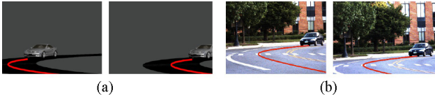
Fig. 3. Examples of curved path constraints for synthetic and actual traffic sequences. (a) Synthetic sequence. (b) Real sequence.
