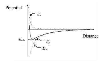
Fig. 6 van der Waals forces generate potential between two protein molecules.
