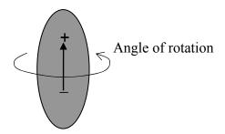
Fig. 8 The protein robot can rotate about its axis of polarized vector which is aligned with the electric field.
