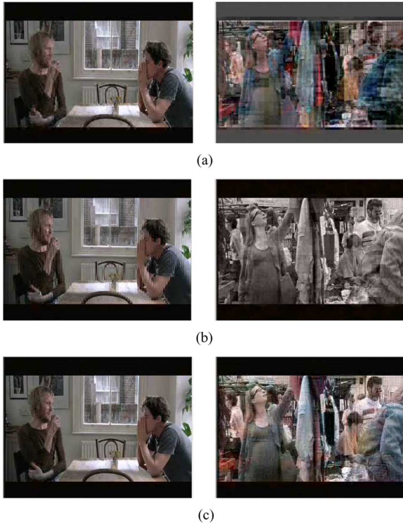
Fig. 9. 1st and 58th reconstructed video frames in Notting Hill (packet loss rate 20%). (a) Conventional UDP/IP without retransmission. (b) Receiver-based retransmission. (c) Content-based retransmission.
