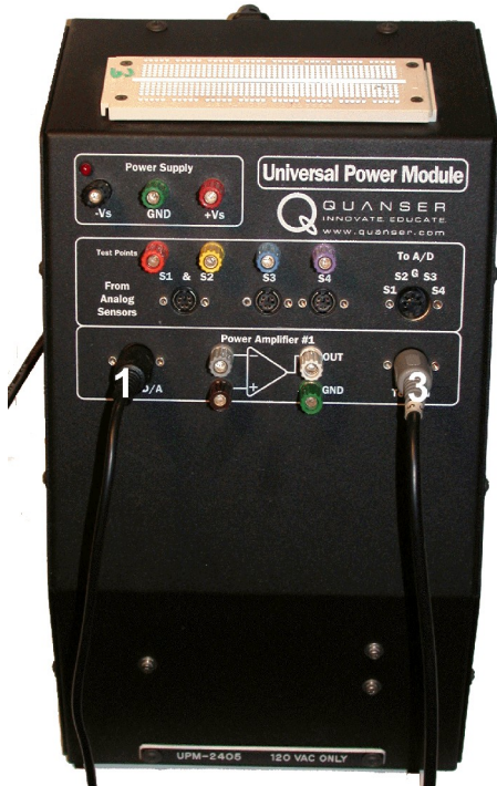
Figure 13: Connection on UPM-2405 for pitch motor.
