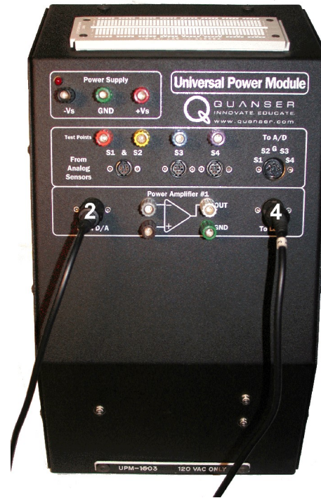
Figure 14: Connection on UPM-1503 for yaw motor.
