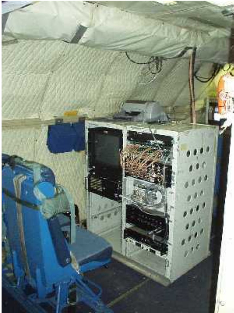
Figure 9: The ESTAR equipment bay.
