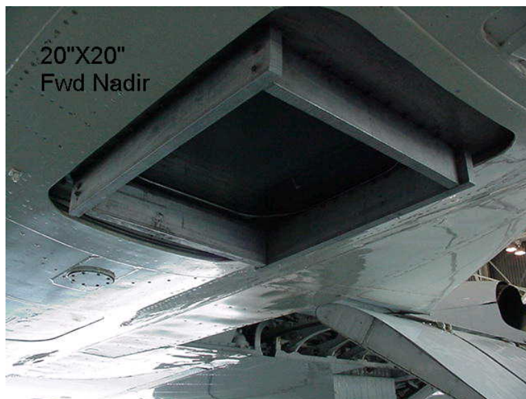
Figure 10: Forward Nadir Optical Port. Located immediately behind the trailing edge of the wings. This port can be accessed via a hatch located a few feet forward of the port (just barely visible in picture). Equipment is mounted on a pair of parallel rails running along the direction of flight above the port. These rails are identical to the ones appearing in the floor of cabin (described in Section 3). Picture courtesy of D. Easmunt, WFF.
