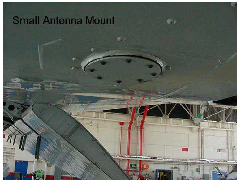
Figure 13: Small mounting point for an external antenna (also visible forward of the optical port shown in Figure 10). At the time of the visit, the nadir-looking antenna for the GPS reflectometry instrument was mounted here. Picture courtesy of D. Easmunt, WFF.
