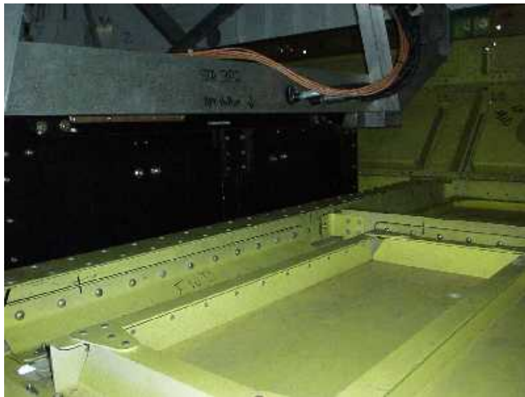
Figure 5: View from just inside open access shown in Figure 4, looking slightly forward. The large black enclosure is ESTAR. The yellow rectangular area in the foreground is the port side half of the nadir facing center access panel. The interior of the bomb bay is 46.5" high. The ribs running along the floor of the bomb bay are 2.5" high.
