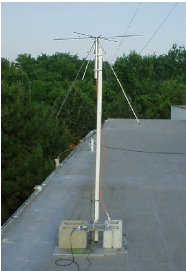
Figure 2: Antenna and front end box, as mounted on the roof of ESL. The antenna is about 10 m above ground level.
