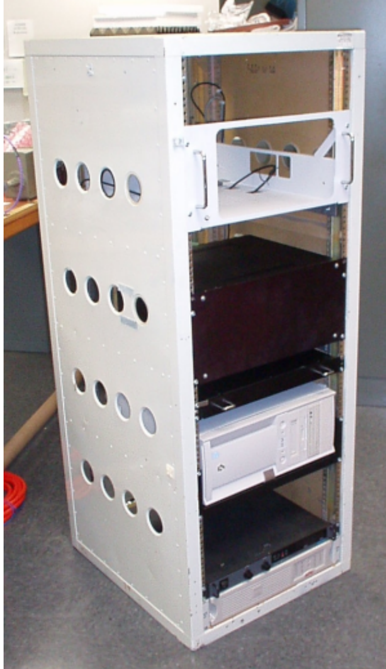
Figure 3: The front of the LISA equipment rack, as it appears when the system is stowed. From top to bottom: Spectrum Analyzer (removed in this picture), LISA electronics box, 1U keyboard/monitor unit, computer, DC power supply, UPS.
