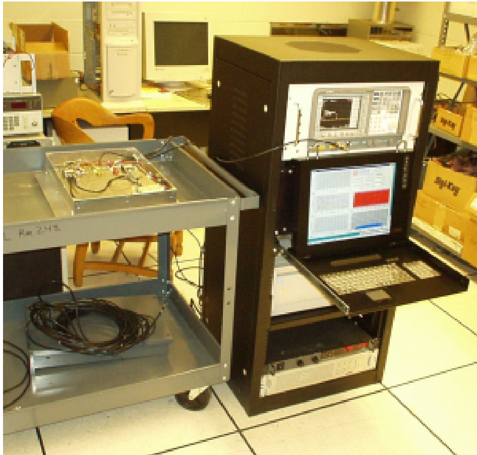
Figure 2: The LISA equipment rack, as it appears when the system is running.
