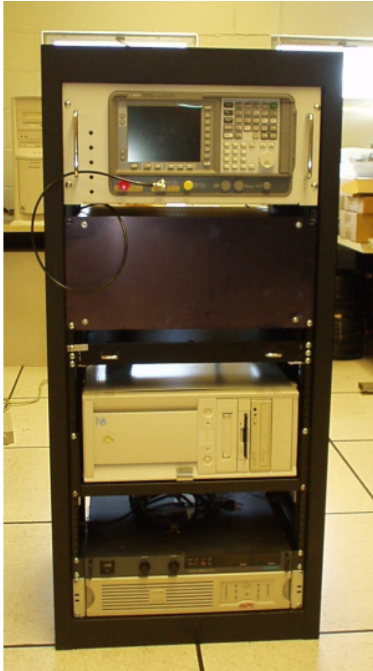
Figure 3: The front of the LISA equipment rack, as it appears when the system is stowed. From top to bottom: Spectrum Analyzer, LISA electronics box, 1U keyboard/monitor unit, computer, DC power supply, UPS.
