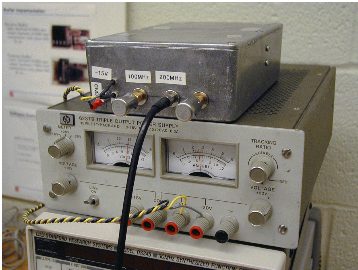
Figure 1: The clock generator module and power supply setup. The generator requires \pm 15V power supply to operate.
