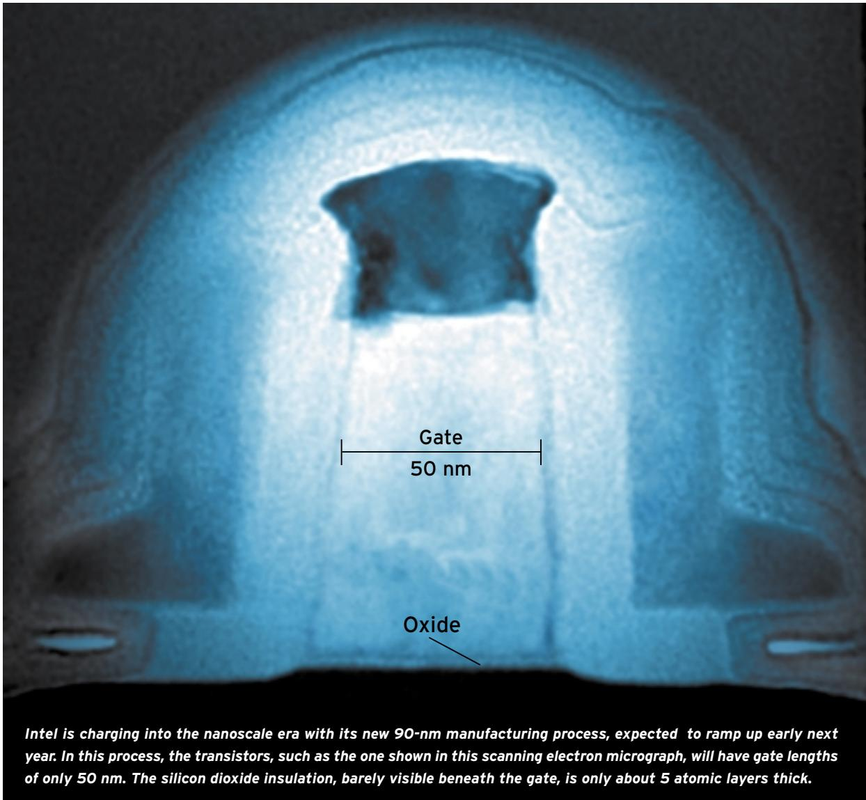
*Intel is charging into the nanoscale era with its new 90-nm manufacturing process, expected to ramp up early next year. In this process, the transistors, such as the one shown in this scanning electron micrograph, will have gate lengths of only 50 nm. The silicon dioxide insulation, barely visible beneath the gate, is only about 5 atomic layers thick.*
