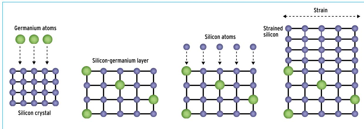
**● Putting a Strain in Silicon to Speed Up Transistors**
