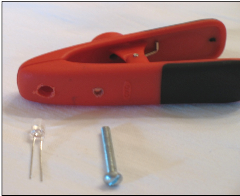
Figure 2. Clip with holes for the placement of the infrared L.E.D. and the pressure adjusting screw.
